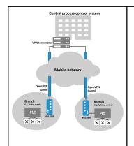
To control their actuators and sensors on site, the REMTEC AG uses a PLC which is connected via Ethernet to the NB1600. Its software supports all common VPN technologies. Thus, the NB1600 can establish an OpenVPN tunnel, which is terminated in the central process control system. Therefore, the incoming and
