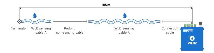
With such a zone, which could be up to 185 meters away from the monitoring device, one could create an effective detection situation by placing the sensing cable right next to the water sources in any type of site, be it a data center, industrial or manufacturing facility, or a warehouse.
