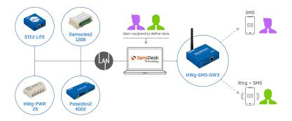
However, both options (SMS-GW unit / SMS alerting from the Portal) have their limitations and advantages. Using gateway unit only can cause a situation, when the monitoring device is turned off (disconnected) - sending a critical alert message
