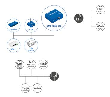
Both 2G (GSM) and LTE (nowadays it's probably not necessary to explain the difference between wireless broadband standards) SMS gateways, named SMS-GW3 as it is the third version of the gateway from our production, serve the same function - to send an alert in the form of a user/device-defined SMS message or to make a call-out alert - which is basically a call to a target phone number.
