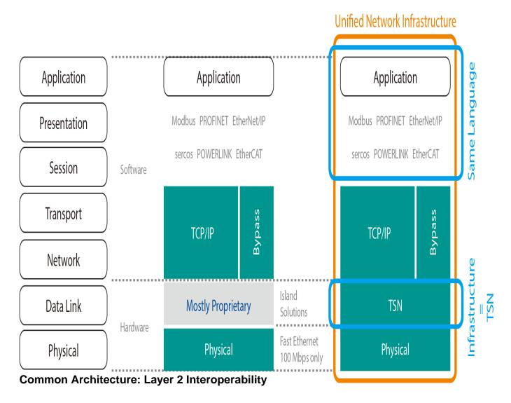
As a deterministic Ethernet standard, TSN is essentially a Layer 2 technology within the Open Systems Interconnection (OSI) model of
